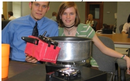
smart pot – maintains temperature in pot at setpoint
