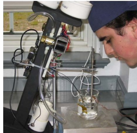
FIGURE 7 ENGR 121 FISHTANK PROJECT DURING CALIBRATION OF RTD.
